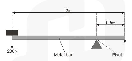
What weight is needed at position *P* to balance the bar?
